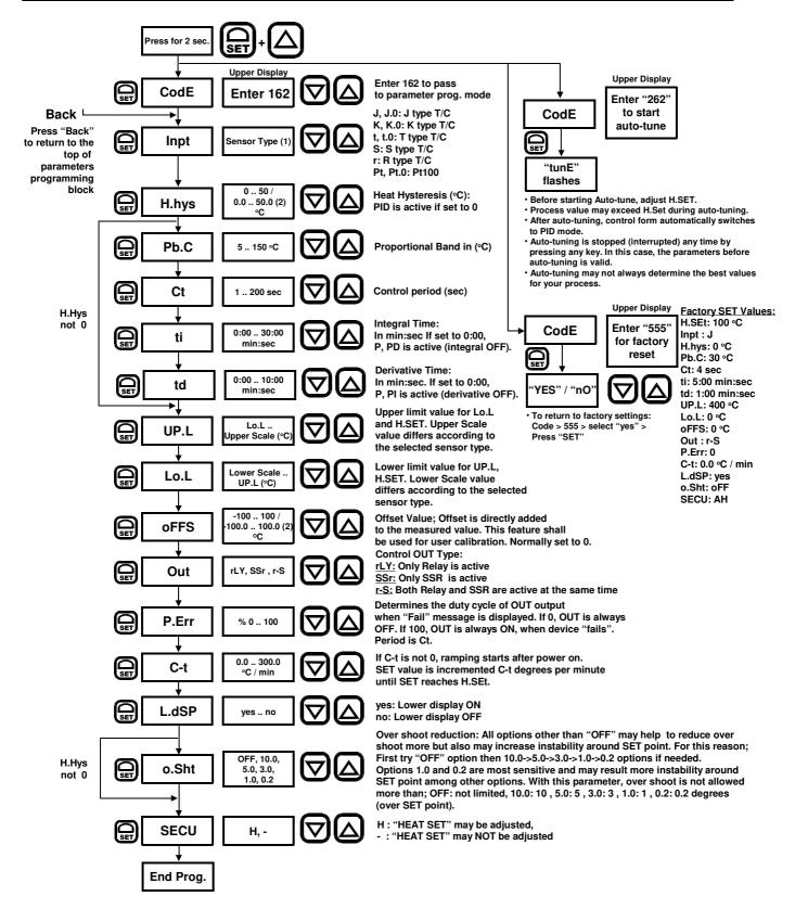
(1) When sensor type is changed, Up.L, Lo.L, H.Set, H.hys, oFFs may be set to a new value automatically, according to the selected sensor.
