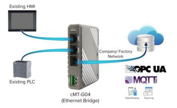
cMT-G04 can be configured by the following ways. Way1. Connect cMT-G04's LAN port with a PC, and on the PC open a web browser and then enter: http://169.254.0.1. password: 111111.
