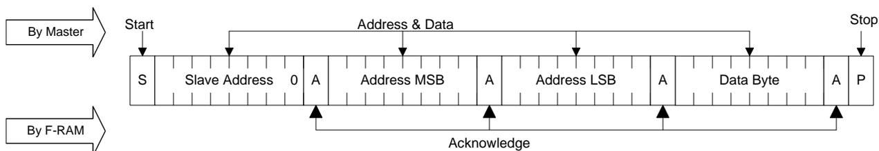
Figure 9. Multi-Byte Write
