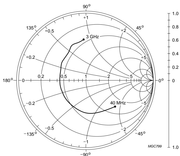
$V_{CE} = 12 \text{ V}; I_C = 70 \text{ mA}; Z_0 = 50 \Omega.$ Fig.11 Common emitter input reflection coefficient ( $s_{11}$ ); typical values.
