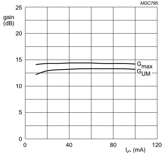
$f = 900 \text{ MHz}; V_{CE} = 12 \text{ V}.$
