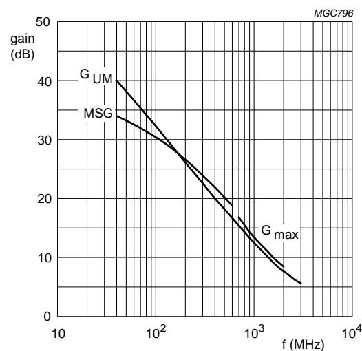
$I_C = 70 \text{ mA}; V_{CE} = 12 \text{ V}.$
