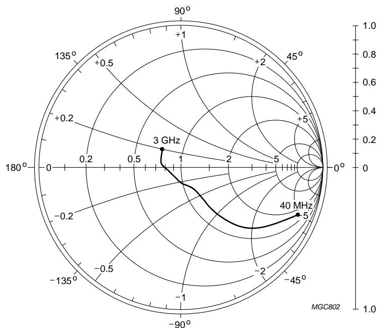
$V_{CE} = 12 \text{ V}; I_C = 70 \text{ mA}; Z_o = 50 \Omega.$ Fig.14 Common emitter output reflection coefficient ( $s_{22}$ ); typical values.
