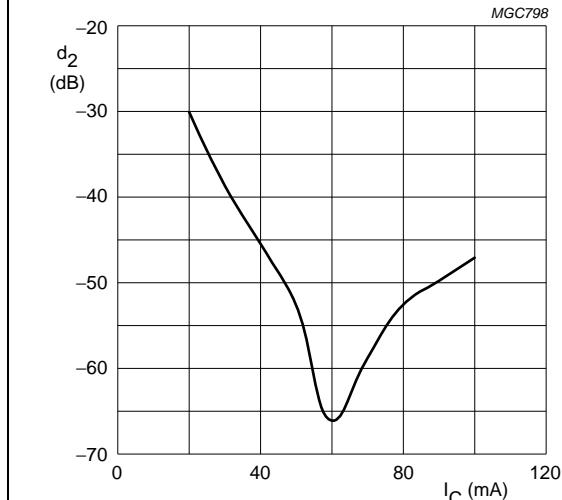
$V_{CE} = 12$  V;  $V_o = 316$  mV;  $f_{(p+q)} = 810$  MHz.
