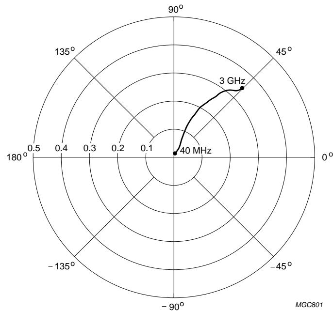
$V_{CE} = 12 \text{ V}; I_C = 70 \text{ mA}.$ Fig.13 Common emitter reverse transmission coefficient ( $s_{12}$ ); typical values.
