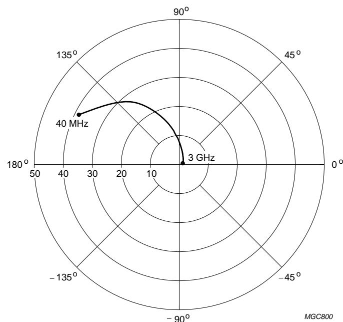
$V_{CE} = 12 \text{ V}; I_C = 70 \text{ mA}.$ Fig.12 Common emitter forward transmission coefficient ( $s_{21}$ ); typical values.
