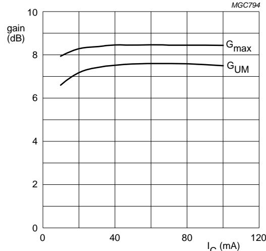
$f = 2 \text{ GHz}; V_{CE} = 12 \text{ V}.$
