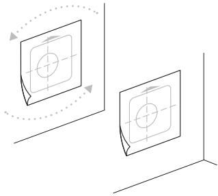
**Attach the mounting template and mark out the area for drilling the duct.**
