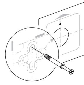
**Drill two mounting holes. Insert the plugs into the mounting holes.**
