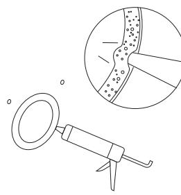
**Fasten the insulation in the duct with a neutral, odorless silicone sealant to form an unbroken loop around the pipe and the internal surface of the duct.**
