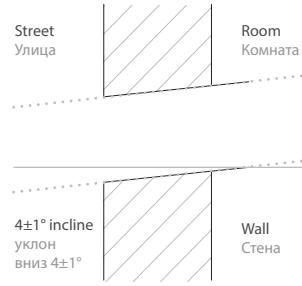
**Drill an air duct with a diameter of 132 mm as shown in the figure.**
