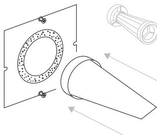
**Install the supplied air filter inside the duct.**
