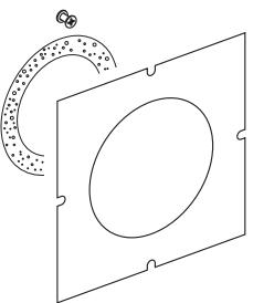
**Stick the sealing element on the wall.**
