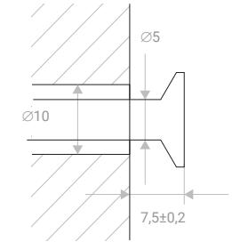
**Screw the self-drilling screws into the plugs. Check that the screw heads protrude from the wall by the amount shown in the figure.**
