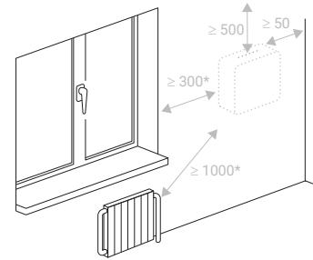
Select a suitable location for the device by following the recommendations in the figure.
