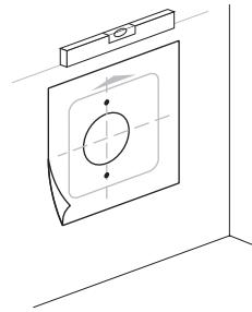
**Align the opening in the template with the air duct. Make sure the template is straight using a spirit level. Mark out areas to drill openings for the fasteners.**
