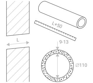
**To heat the duct, we recommend using a polyethylene foam pipe with an internal diameter of 110 mm and a wall thickness from 9 to 13 mm. Cut the pipe to a length slightly bigger than the thickness of the wall.**
