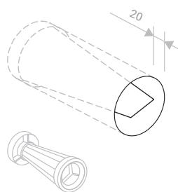
**The side of the filter facing the room should extend at least 20 mm into the duct.**
