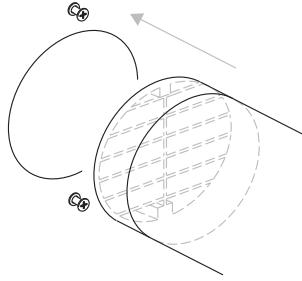
**Install insulation on the air duct with the intake grille facing outward. The veins of the grille should be directed downwards.**
