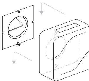
**Put the device power cable into one of the ducts on the rear panel and hang the device on the screws.**
