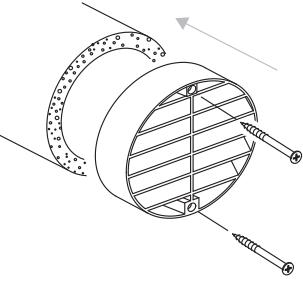
**Fasten an air-intake grille with a diameter of no more than 130 mm to the end of the pipe.**
