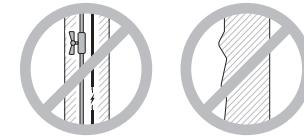
The wall design must allow for the drilling of a ventilation duct. There must be no pipes within the walls at the drill site.
