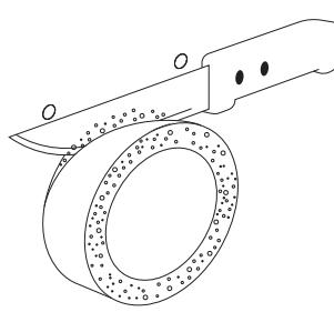
**Cut the insulation to the same size as the surface of the wall.**
