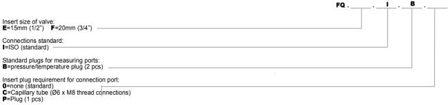
Example: FQ.E.I.B.0=15mm FlowCon QuickDisc™, female-female ISO with 2 p/t plugs and no plug for connection port.
