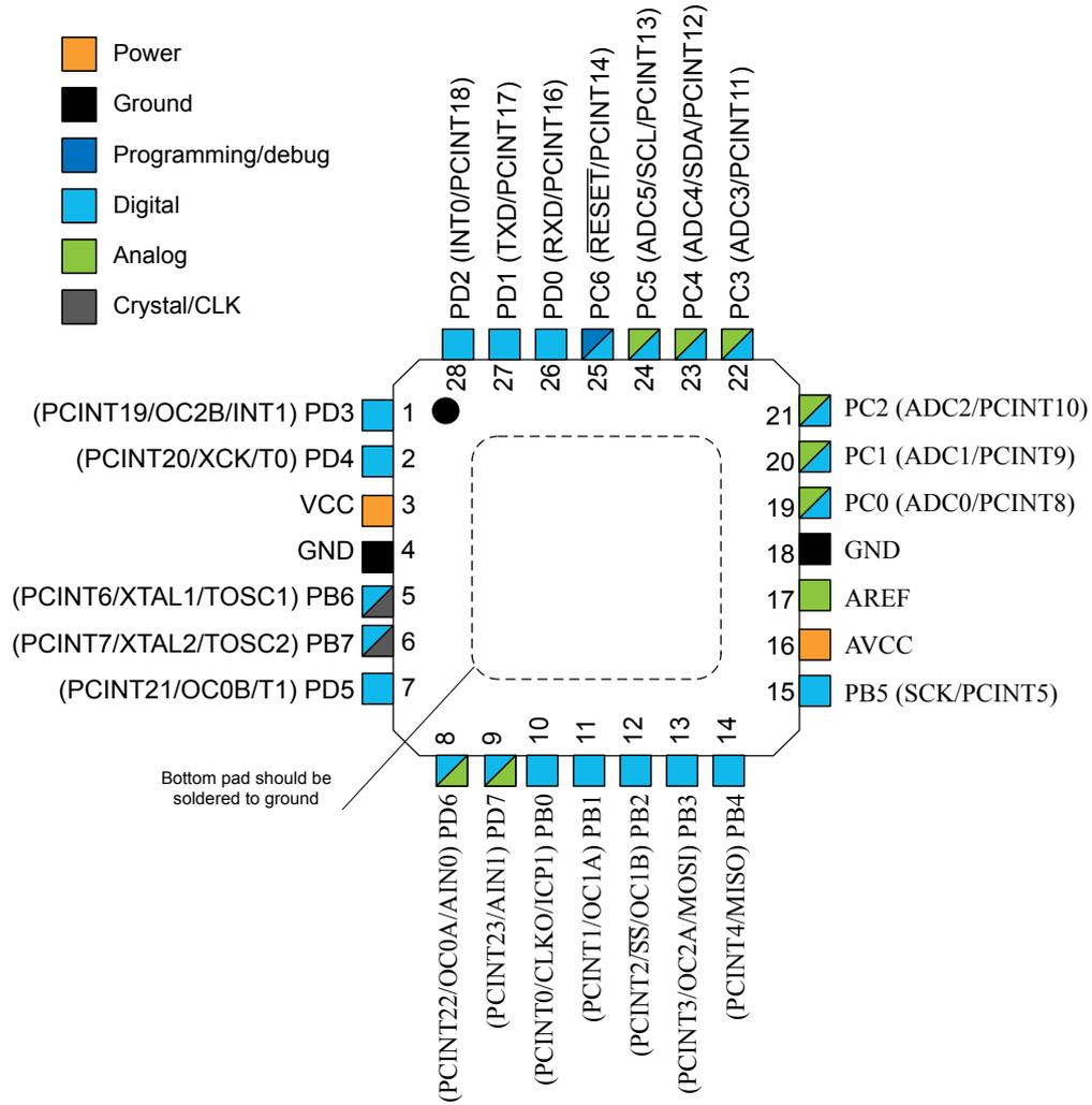
Figure 5-3. 32-pin TQFP Top View
