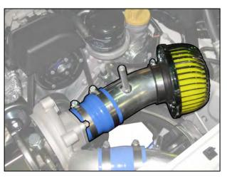
(5) Extend the ventilation hose using the 12mm hose union and supplied rubber hose. Connect the extended hose to the Air Intake Tube.
