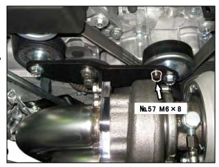
(2) Install the Turbine Heat Shield by sliding the cut outs over the down pipe hardware as shown in the photo.
