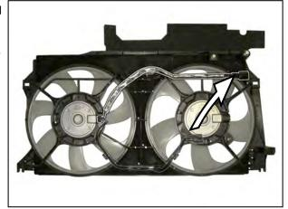
(3) Reinstall the radiator fan, radiator fan shield, reservoir tank and reconnect the radiator fan harness coupler.
