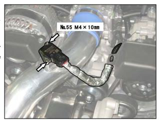
(4) Connect the Compression Tube and Free Rotation Union to the Turbo Actuator.
