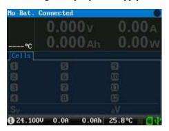
When it is not Regenerative discharging, the icon 'D' on the left bottom is grey; When it is Regenerative discharging, the icon turns to green
