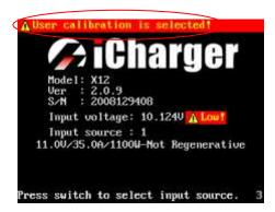
Note: User Calibration has *Channel Calibration* and *Other Variables Calibration* two options, users can calibrate charger for one channel alternatively. If user selects *User Calibration*, the corresponding message will appear in the interface after booting the charger, as shown in the right picture above.
