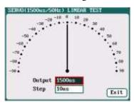
Liner Test: When turning the knob, the pointer deflects with the setting value of Step, and the servo responds accordingly.
