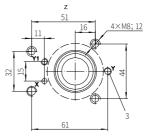
Valve fixing screw M8x40-10.9 grade GB/T70.1-2000
