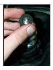
STEP 38. Install reverse lockout spring.
