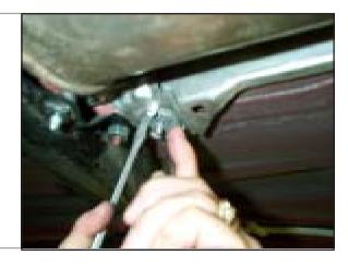
STEP 3. Loosen exhaust coupling bolts.
