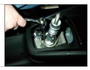
STEP 32. Install retaining clip removed in step 16.
