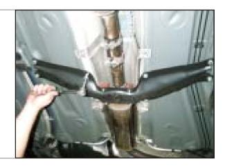
STEP 52. Slide exhaust coupling back over both pipes.
