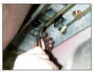
STEP 11. Remove retaining clip from shift linkage.
