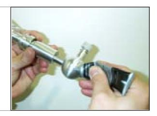
STEP 24. Insert nylon pivot cup into shift mechanism.
