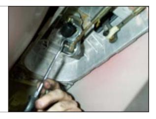
STEP 10. Pry cable off of shifter.
