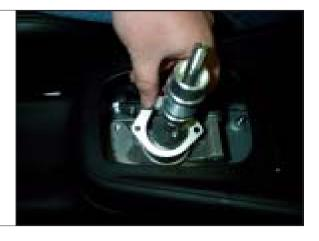
STEP 31. Tighten two (2) reverse lockout plate bolts.
