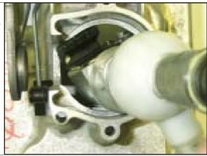
STEP 21. Remove knob/boot assembly from shifter.
