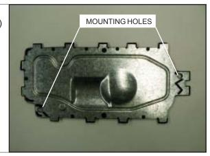
STEP 48. Reinstall front heat shield.
