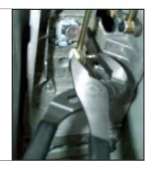
**STEP 46.** Reinstall retaining ring onto shifter.
