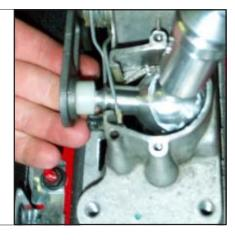
**STEP 25.** Set return spring into corresponding groove on pivot arm. Tool: Screwdriver (flat)
