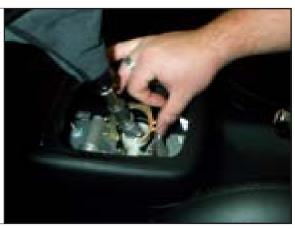
STEP 19. Pull stick upward and remove pivot bushing.
