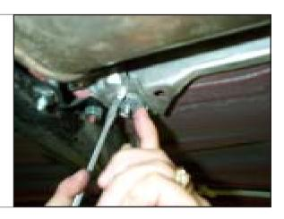
STEP 51. Reinstall center exhaust support.
