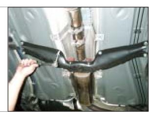
STEP 7. Remove center heat shield.
