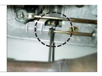
**STEP 12.** Remove cable from shift linkage.
