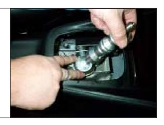
STEP 28. Thread set screw with nylon slider into reverse lockout plate until nylon is fully seated against plate.
