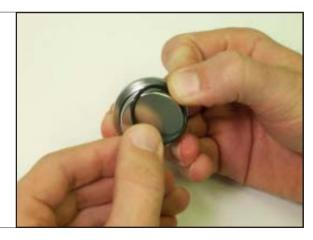
STEP 41. Install insert into knob.
