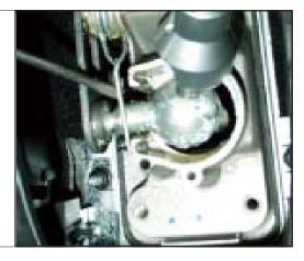
STEP 26. Install plastic pivot bushing on B&M Short Throw Shifter.
