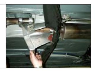
STEP 8. Carefully pry bottom plate off of shifter enclosure.
