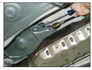
STEP 9. Remove retaining clip from shifter. Tool: Screwdriver (flat)
