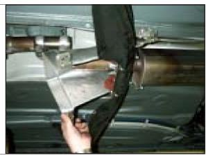
STEP 50. Reinstall heat shield snap washers.
