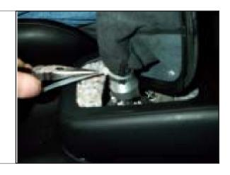
STEP 36. Install shift boot into center console.
