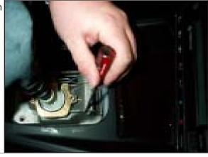
STEP 17. Remove bolts securing top plate.
