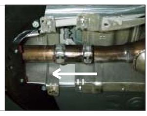
STEP 53. Tighten bolts on coupling.
