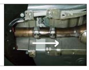
STEP 5. Remove front heat shield.
