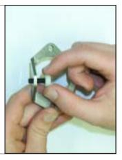
STEP 29. Install and tighten jam nut on slider set screw.
