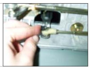
STEP 45. Install cable onto shifter.
