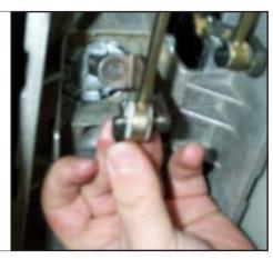
STEP 47. Reinstall bottom plate on shifter enclosure.
