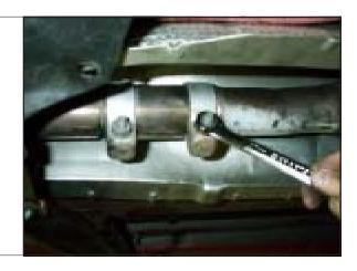
**STEP 4.** Slide exhaust coupling forward.
