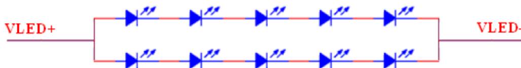
Figure 4.2 LED connection method
