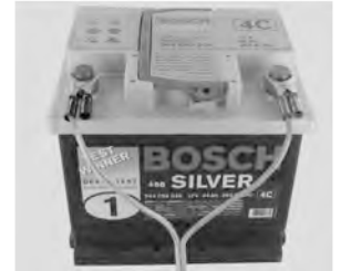
Using terminal clip attaching to car battery
