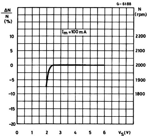
**Figure 20:** Speed Variations vs. Motor Current (MOTOR)
