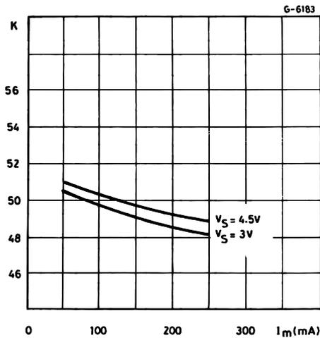
**Figure 18:** Saturation Voltage vs. Load Current (MOTOR)
