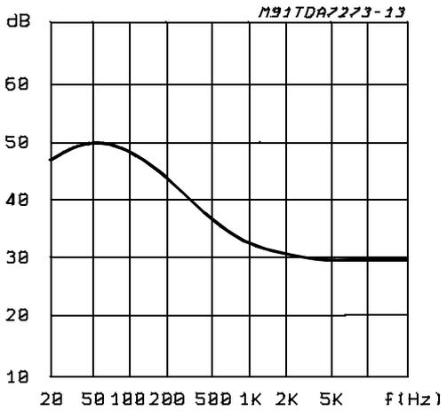
**Figure 6: Distortion vs. Frequency (PREAMPLIFIER)**
