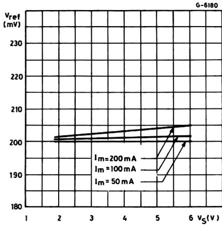
**Figure 16:** Shunt Ratio vs. Supply Voltage (MOTOR)
