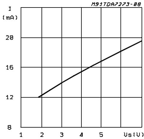
**Figure 4: Reference voltage Vs/2 (pin 20) vs. Supply Voltage**
