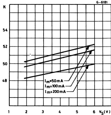
**Figure 17:** Surt Ratio vs. Load Current (MOTOR)
