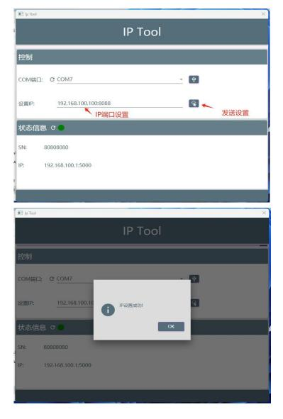
5. Restart the device and reconnect to the IP tool software. You can find that the IP has been modified.
