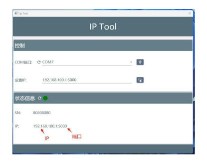
4. Set the IP and port as follows: enter the IP we want in the set IP to and port, the format is: IP number: Port number, for example: 192.168.100.100:8088 Click the Send settings button later. The words "Set IP successfully" appear.
