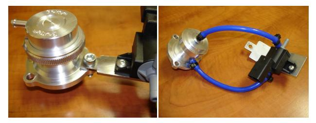
With the new Forge valve loosely mounted to the turbo, and a location selected for the solenoid and it loosely mounted as well, measure to find appropriate lengths for the vacuum hose connections between the valve and the solenoid.
