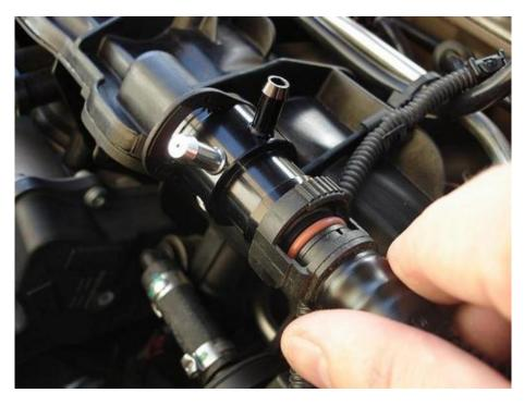
From the appropriate nipple on the manifold tap (largest port), run a length of vacuum tubing along the top of the motor, around the passenger side, following the fuel rail and fuel lines, down to the remaining linear port on the solenoid you mounted previously. (See plumbing diagram) Secure both ends of this line using two of the included zip ties. If any spare zip ties are available, use them to secure this vacuum line to the fuel rail and/or fuel lines.
