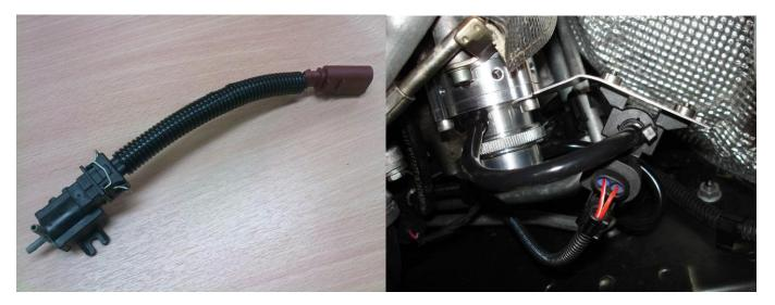
With the valve securely mounted to the turbo and the solenoid bracket also secured at your desired location within the engine bay, you can reconnect the OEM wiring harness plug to the connection on the end of the Forge wiring harness.
