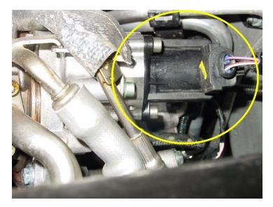
Once located, disconnect the electrical connector/plug for the valve and you can now use your 5mm Allen wrench or socket to remove the three 5mm Allen bolts which secure the valve to the turbo. <u>You must be sure to save the OEM valve bolts as they will be reused later.</u>
