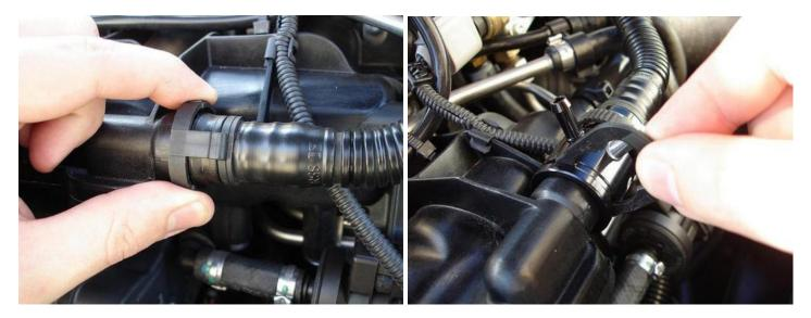
Once the manifold tap is held securely in place with the plastic C-clip, reattach the PCV hose to the barb at the end of the tap. If you are using some sort of PCV "fix" or "bypass", however, you will need to reconnect whatever components are supplied with that product. The barb on the end of our manifold tap is the same size and shape as the OEM manifold barb, so any hoses or caps that connect to the manifold barb will connect to the barb on our tap as well.
