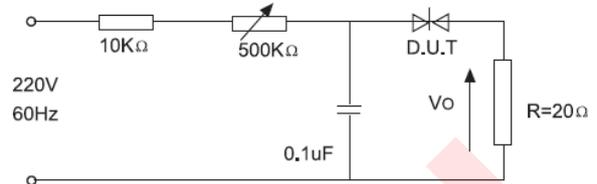
FIG.3-TEST CIRCUIT SEE GIF.2 ADJUSTR FOR  $I_p=0.5\text{A}$
