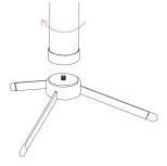
**Please note:** the M8 threads are not designed for several tubes to be screwed together to form one long tube element.
