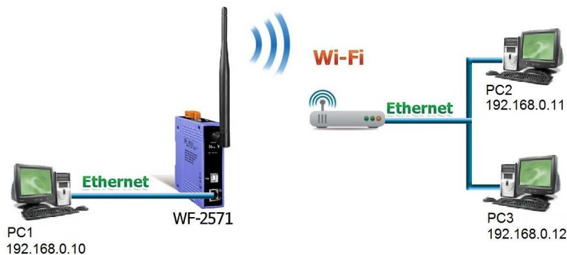
Figure 4-8: AP connection test architecture
