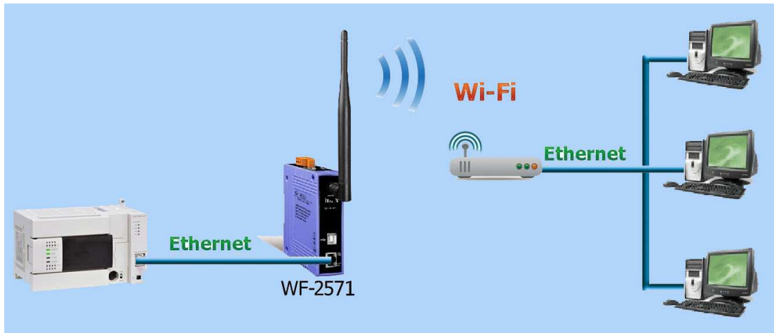
Figure 1-1: Application architecture for the WF-2571
