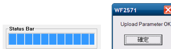
Figure 4-3: Parameter transmission status and upload successful screens
