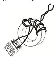
Wire the 24 VAC supply power wires from the transformer to the HOT and COM terminals on the terminal plug as shown in the following figure. The middle terminal on the supply power terminal block is not used. See Table 4 for more information about the Supply Terminal Block.
