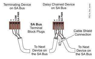
Stranded, 4-Wire (2 Twisted Pair) Shielded Cable (One twisted pair is the + and - leads.
