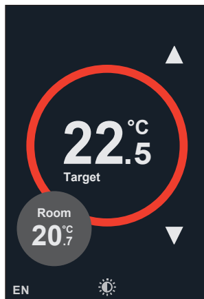
Fig. 8a Language abbreviation (opens by tapping the selection of the language options)
