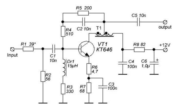
Transformer T1 assembled on toroid 10x6x5. Wire: 0.35 mm, 5 turns by two twisted wires. The end of the first wire should be connected to the beginning of the second wire (pin 2).
