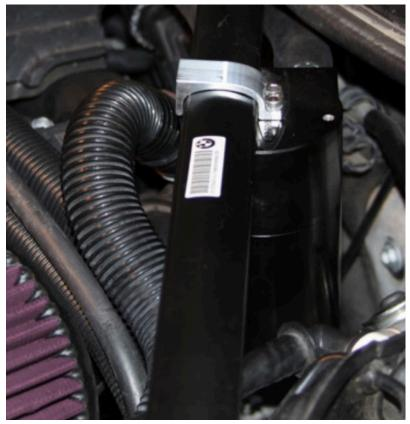
Holding the DV line out of the way swing the OCC under the strut brace and attach using the included allen screws and bracket. Only one screw is required to hold the OCC up but both can be installed.
