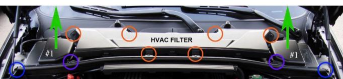
Now remove the sensors circled in purple in the above photo. Some vehicles have 1, some have 2 sensors. Turn clockwise to loosen. Pull up on the tabs holding the wires going to the sensors and set them aside.
