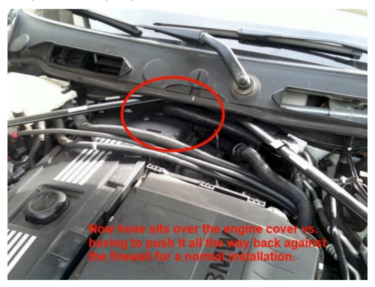
Once the engine cover is installed you can reinstall the cowl and cabin filter. Installation is complete!
