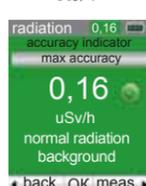
Accuracy indicator bar is intend to display the current level of items accuracy. As more it filled, as more item is accurate. Bar is filling first with green then yellow and red line. Finally, the accuracy bar will be replaced with "max accuracy" phrase. That means that item is now displaying the most accurate result.
