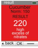
When the measurement is complet item will display numeric result and one of three possible working messages.
