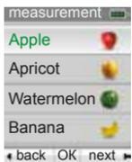
In the "Measurement" menu choose measuring product from the list and press "OK" button. To return to the main menu, press left arrow button on the keyboard.
