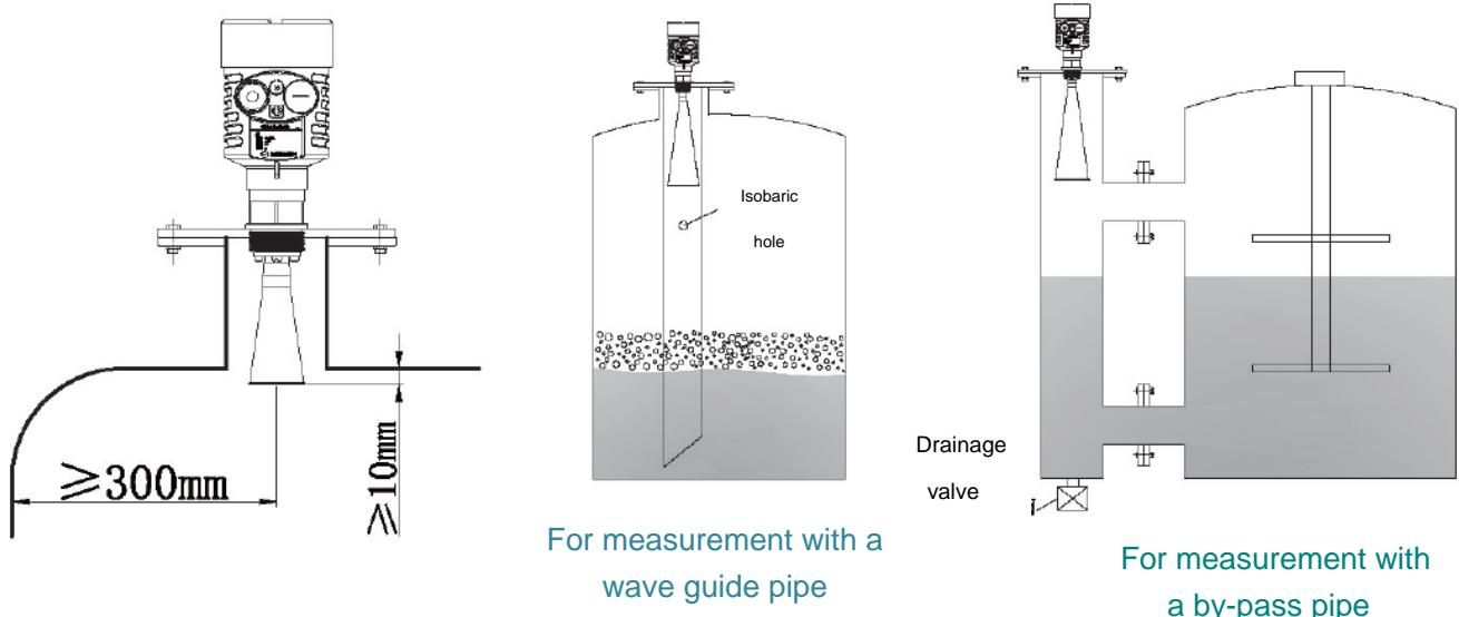
The minimum distance between the symmetrical central line of the transmitter and the inner tank wall should be at least 300mm
