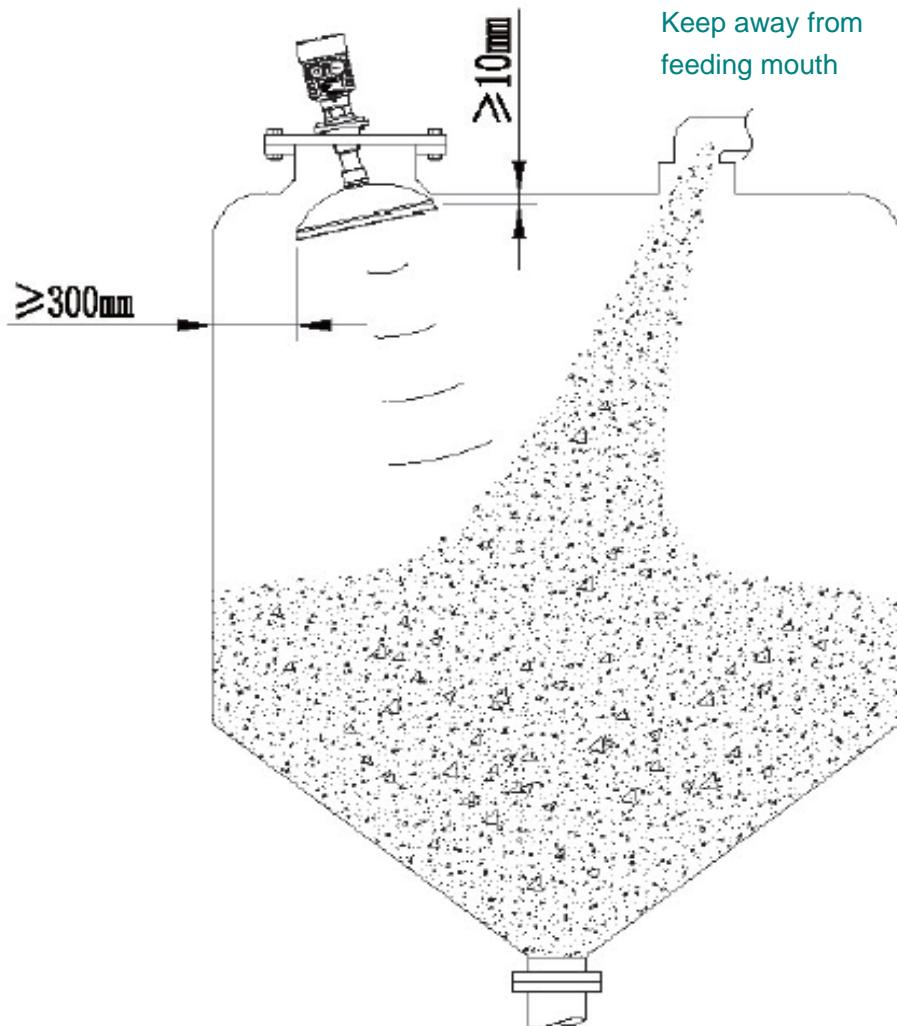
The minimum distance between the outskirt of the parabolic antenna and the inner tank wall should be at least 300mm
