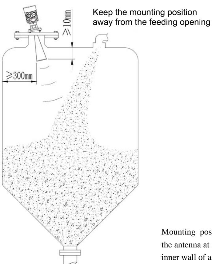
Mounting position: keep the outskirt of the antenna at least 300mm away from the inner wall of a tank
