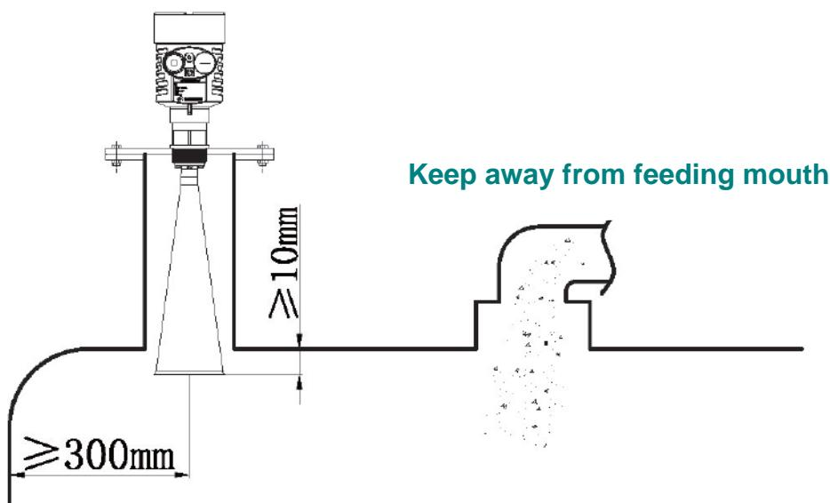
The minimum distance between the symmetrical central line of the transmitter and the inner tank wall should be at least 300mm
