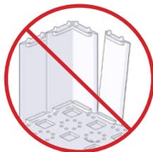
Make sure to straighten walls and then loosely apply modules on top so pegs and holes align before squeezing together.
