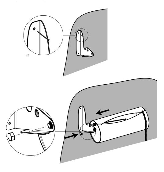
3) Install the axis on the opposite side of the body **A** into the orifice in the second wall bracket **F**. Make the locknut **B** onto the device's axis. Fix the wall bracket **F** on the wall.
