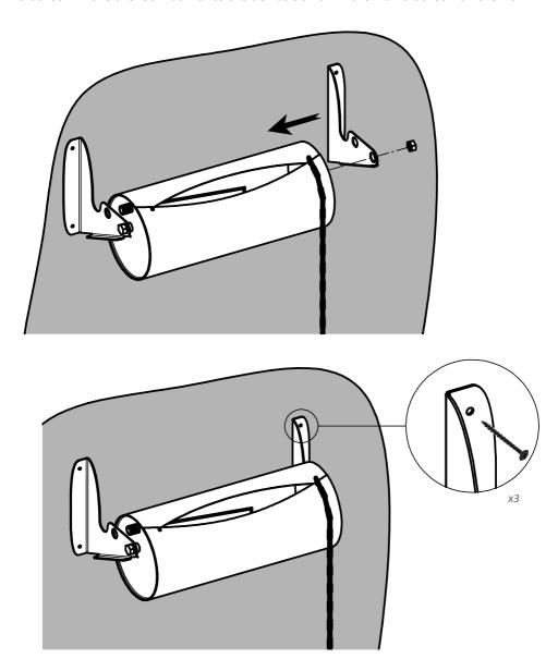
Note: the assembly and installation procedure for a wall-mounted device is described above. The procedure for mounting on the ceiling is similar except that the body axis  $\bf A$  is installed into the holes at the base of the wall brackets  $\bf F$ .
