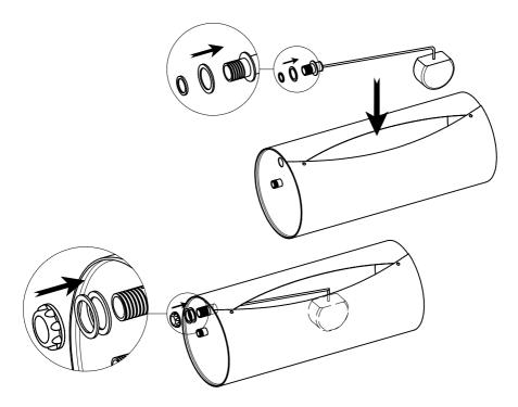
2) Install the chain with handle **D**, and fix it using a winged nut **E**.
