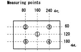
TOPCON BM-7 + quartz fiber Measureing spot size :  $\phi$  10 mm
