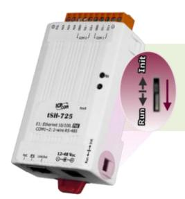
Step 11: Once the update is complete (i.e., when the progress indicator reaches 100%), set to "Run Mode".
