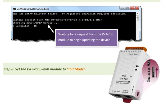
Step 9: Power-on reset the tSH-700 RevB module in "Init Mode" to initiate the update.
