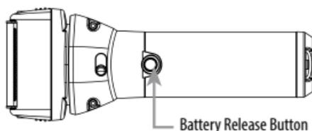
2. The battery will partially eject but needs to be pulled from the bottom of the shaver to remove completely.
