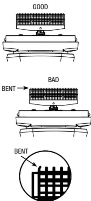
Always check to be sure the cutters are not bent in any way.
