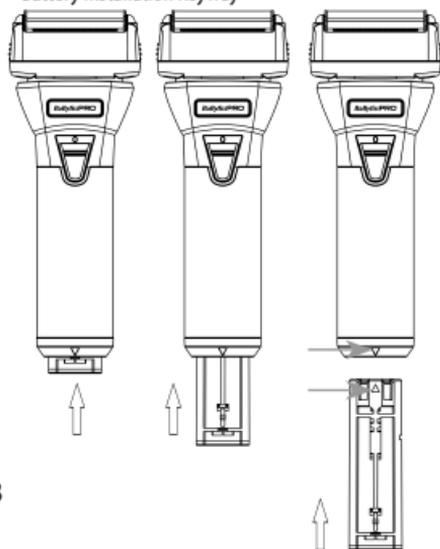
**WARNING** - Make sure the shaver and battery are aligned properly before pushing battery all the way in. Do not force battery in if any resistance is felt.
