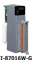
2-channel Isolated Strain Gauge Input Module
