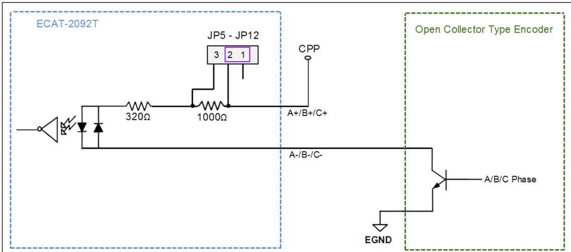
Figure 8: Open collector wiring diagram (Source Digital Input)
