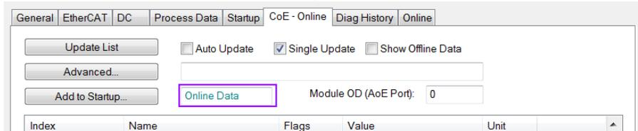
**Step 2:** Do all the necessary configuration by entering the correct parameter values for the configuration objects (0x8000, 0x8010). The setting is being done by double clicking the configuration parameter and selecting an option from the shown drop list box. In the following picture the signal polarity of the A signal of encoder channel 0 is being set.
