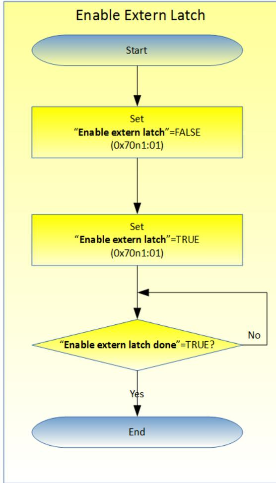
Figure 33: Activating external HR latch
