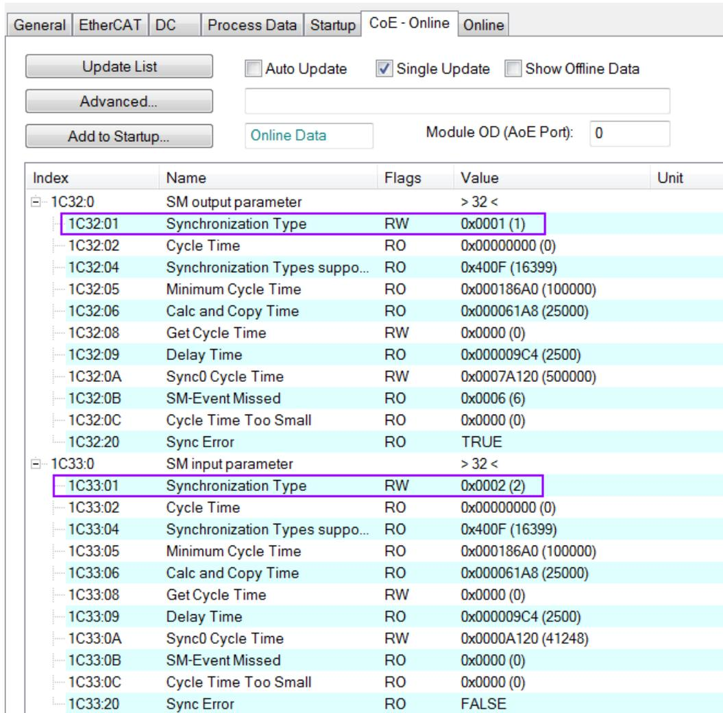
Figure 16: SyncManager setting for Free-Run mode
