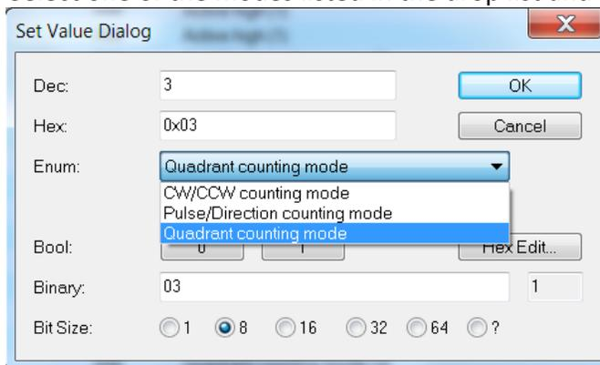
**Step 3:** Once the setting has been successfully sent to the slave it will be displayed in the CoE online parameter list. In the figure below "CW/CCW counting mode" has been selected for channel 0. This value needs only to be set once and therefore does not have to be sent in every cycle time.
