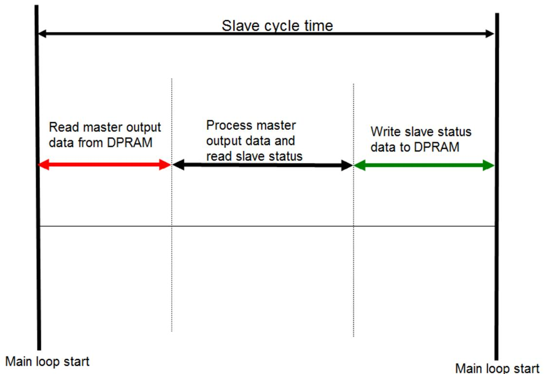
Figure 15: Slave processing sequence in Free-run mode
