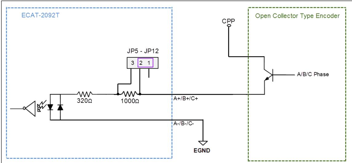
Figure 9: Open collector wiring diagram (Sink Digital Input)
