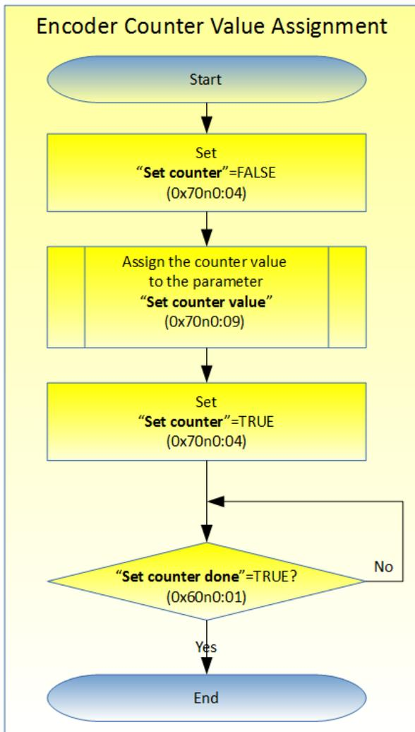
Figure 32: Encoder counter setting
