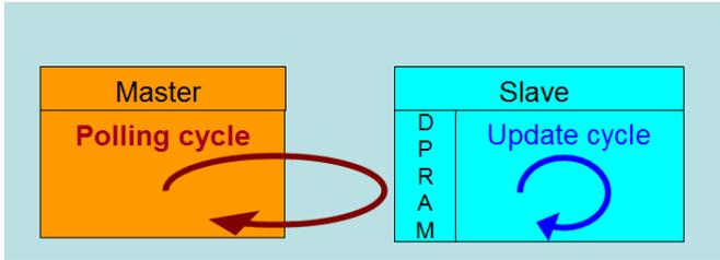
Figure 14: Master-slave cycle in Free Run mode
