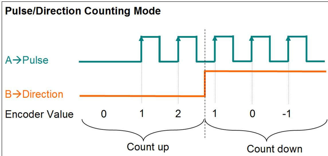
Figure 28: Pulse/Direction counting mode
