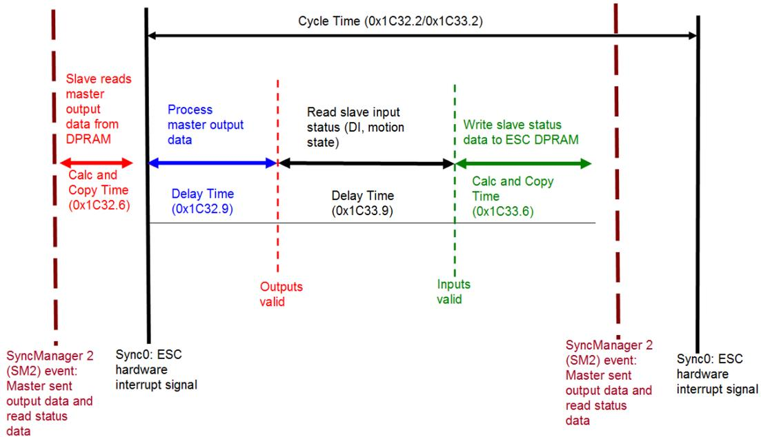
Figure 19: Internal slave processing sequence in DC mode
