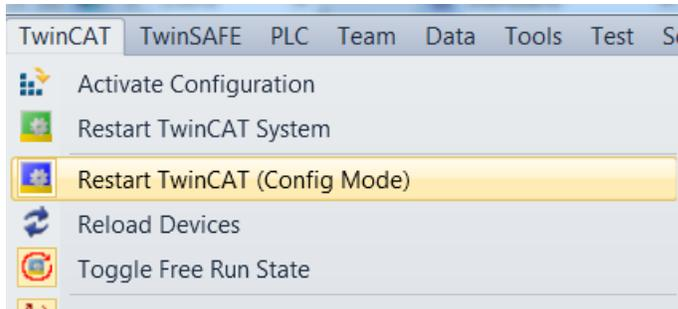
Figure 26: Download PDO assignment and restart TwinCAT
