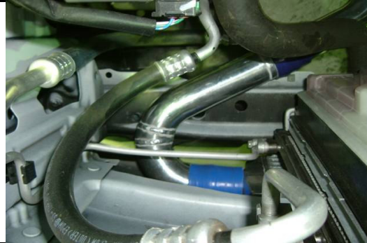
Oil Drain ( To Oil Pan)
