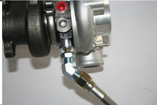
Oil Drain ( To Oil Pan)
