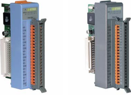
I-87068 I-87068-G 8-ch Power Relay Module (5A Rating Current)
