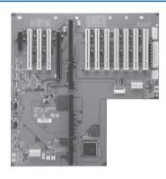
PICMG 1.3 ① PCI 10 PCIe x4 1 PCIe x16 1
