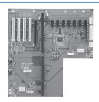
PICMG 1.3 ① PCI ④ PCle x1 PCle x16
