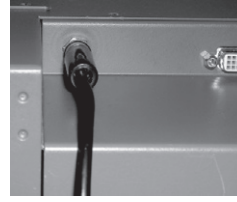
▲ Screw-type power input
