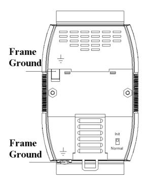
New DIN rail models are available that can easily be connected to the earth ground. Each is made of stainless steel, which is stronger than those made of aluminum. There is a screw at one end and a ring terminal is included as shown in the figure below. Refer to Section 1.11.1 for more information about the new DIN rail models.
