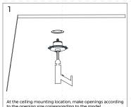
At the ceiling mounting location, make openings according to the opening size corresponding to the model.
