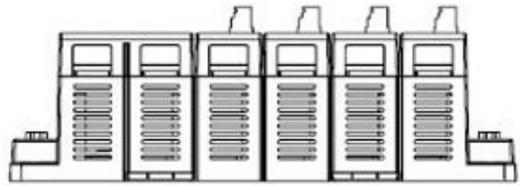
Using DIN rail clips or Screw poles around the corners allows the control unit to be easily mounted on the control box
