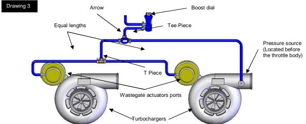
\*Note for sequential turbo systems: Sequential turbo setups can be complex and vary from car to car. Please contact your local Turbosmart dealer for more details
