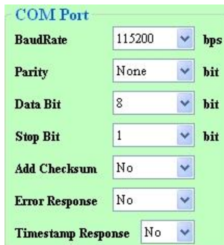
Figure 3-10: The COM port of I-7530A-MR configuration.
