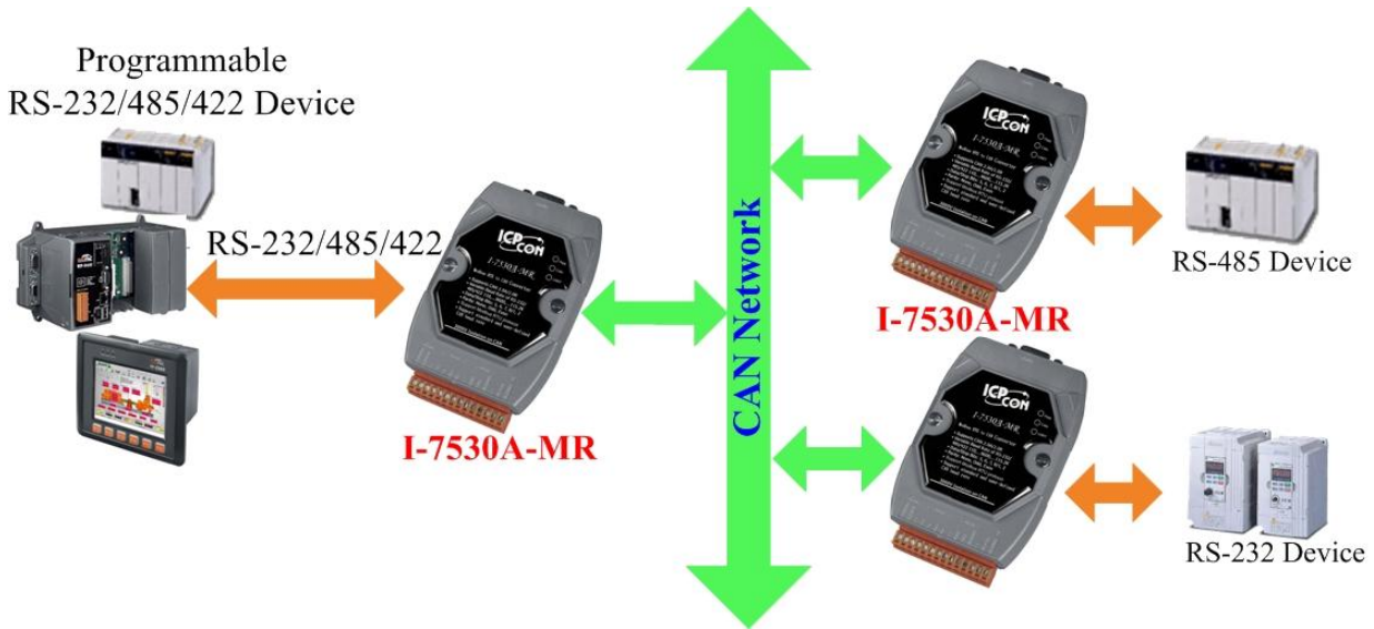
Figure 1-2: The application architecture in the pair-connection mode.
