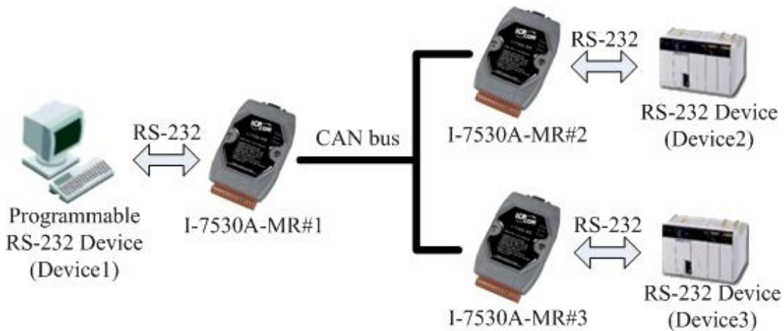
Figure 3-24: The diagram of Application 3.
