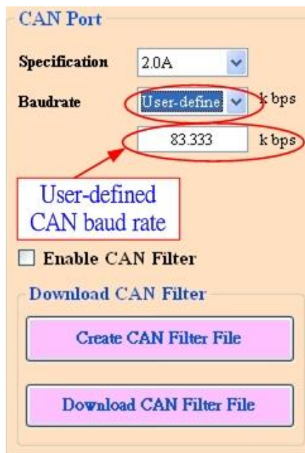
Figure 6-1: User-defined CAN Baud Rate for I-7530A-MR
