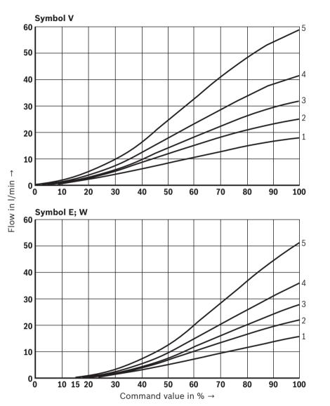
**Rated flow 16 l/min** ( $P \rightarrow A$ ;  $B \rightarrow T \text{ or } P \rightarrow B$ ;  $A \rightarrow T$ )
