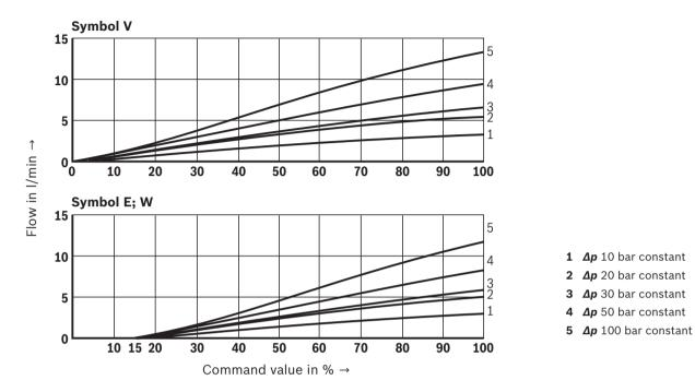
**Rated flow 8 l/min** ( $P \rightarrow A$ ;  $B \rightarrow T \text{ or } P \rightarrow B$ ;  $A \rightarrow T$ )
