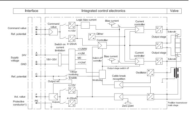
1) PE is connected to the cooling body and the valve housing
