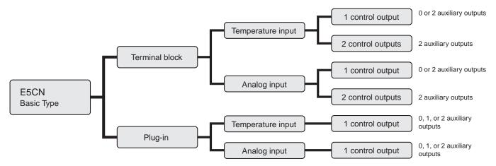
Note: Models with one control output and one or two auxiliary outputs and models with two control outputs can be used for heating/cooling control.
