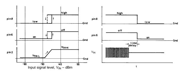
As shown above, when input level is raised and the pin 2 voltage reaches the  $V_{TH-H}$  level of the comparator, pins 6 and 8 turn over. ( $V_{IN} = -45 \text{ dBm}$ ).
