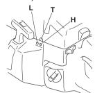
The L and H-jets are used to adjust the supply of fuel to match the rate that air is admitted, which is controlled with the throttle. If they are screwed clockwise the air/fuel ratio becomes leaner (less fuel) and if they are turned anti-clockwise the ratio
