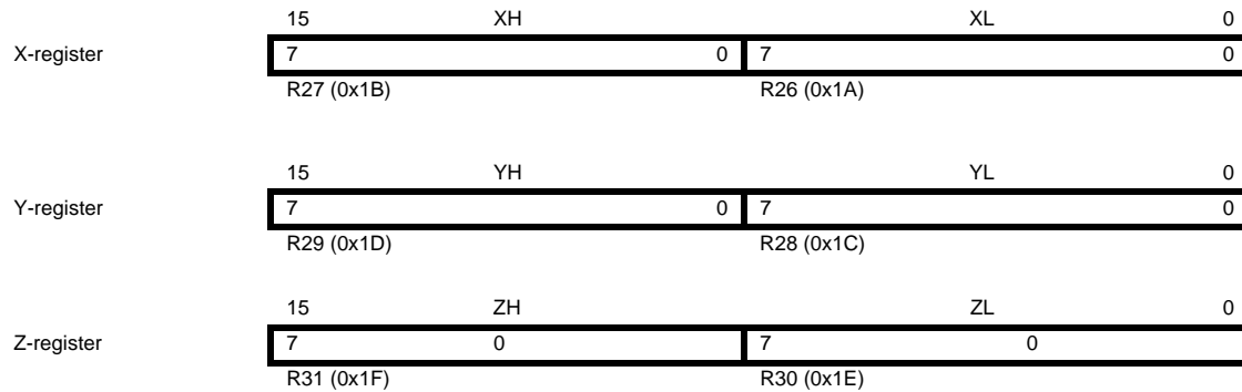
Figure 4-3. The X-, Y-, and Z-registers
