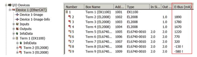
Fig. 12: System manager current calculation
