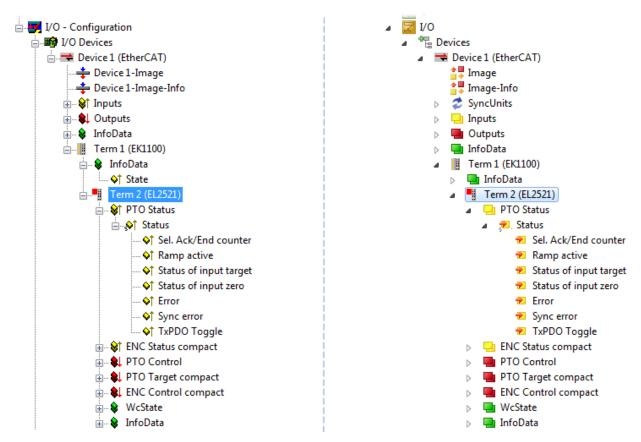
Fig. 100: EtherCAT terminal in the TwinCAT tree (left: TwinCAT 2; right: TwinCAT 3)
