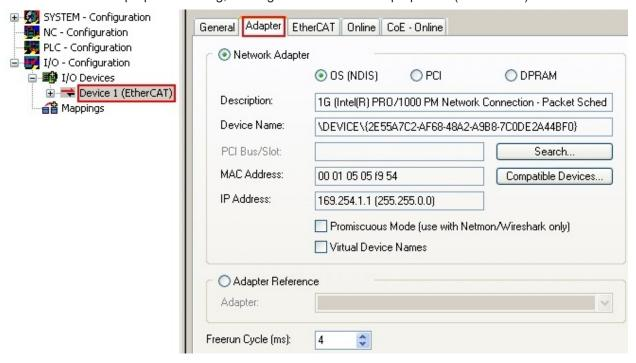
Fig. 94: EtherCAT device properties (TwinCAT 2)
