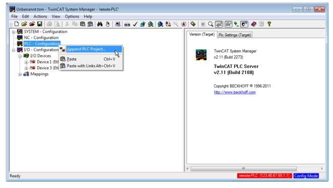
Fig. 44: Appending the TwinCAT PLC Control project
