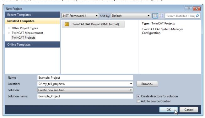
Fig. 53: Create new TwinCAT project
