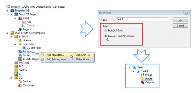
Fig. 144: Insertion of a free task
