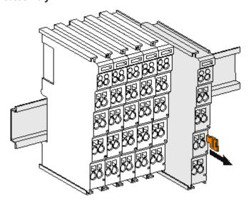
Fig. 21: Disassembling of terminal
