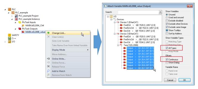
Fig. 68: Selecting several PDOs simultaneously: activate "Continuous" and "All types"
