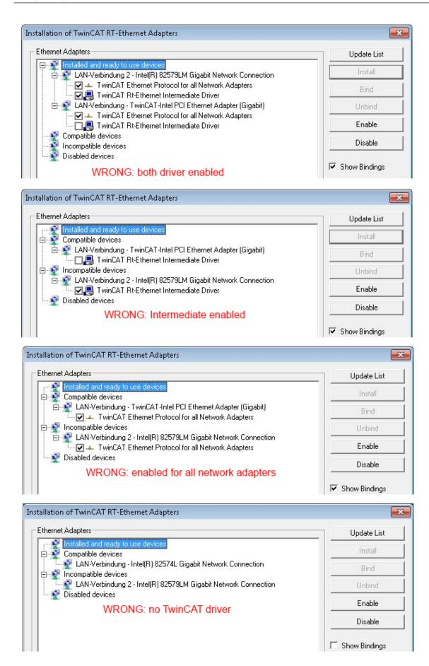
Fig. 81: Incorrect driver settings for the Ethernet port
