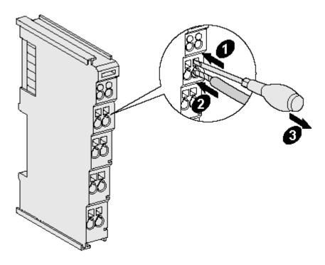
Fig. 26: Mounting a cable on a terminal connection
