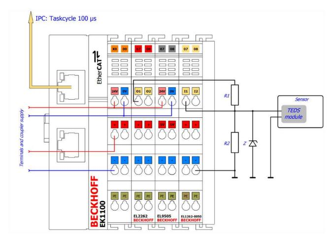
Fig. 189: Wiring for sample program 3
