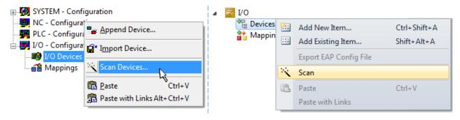
Fig. 102: Scan Devices (left: TwinCAT 2; right: TwinCAT 3)
