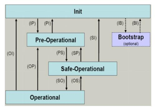
Fig. 14: States of the EtherCAT State Machine
