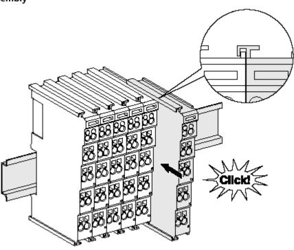
Fig. 20: Attaching on mounting rail
