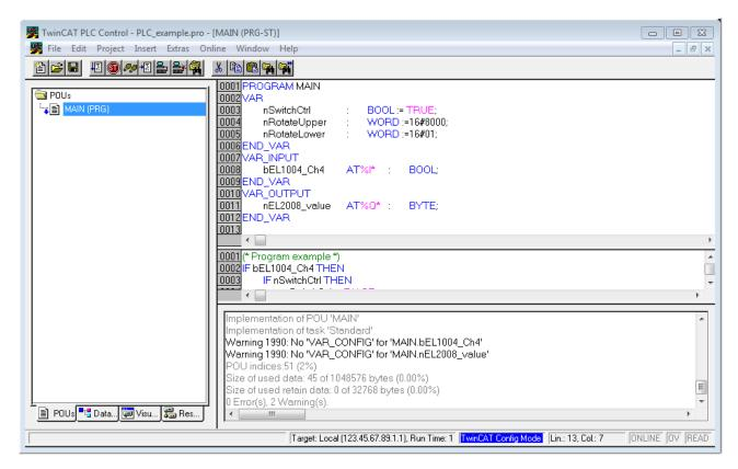
Fig. 43: Sample program with variables after a compile process (without variable integration)
