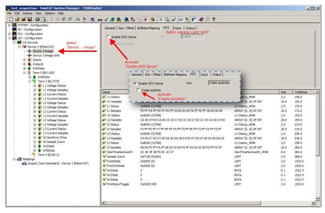
Fig. 167: Activation of the ADS server of the EtherCAT Device (TwinCAT 2)
