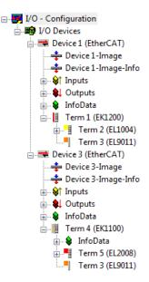
Fig. 40: Mapping of the configuration in the TwinCAT 2 System Manager
