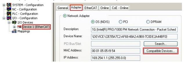
Fig. 78: EtherCAT device properties(TwinCAT 2): click on "Compatible Devices..." of tab "Adapte""
