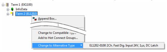
Fig. 121: TwinCAT 2 Dialog Change to Alternative Type
