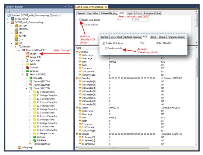
Fig. 152: Activation of the ADS server of the EtherCAT device (TwinCAT 3)
