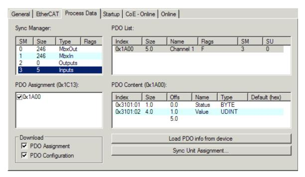
Fig. 125: "Process Data" tab
