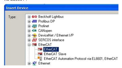
Fig. 92: Selecting the EtherCAT connection (TwinCAT 2.11, TwinCAT 3)
