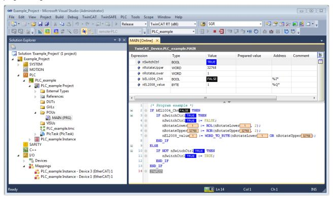
Fig. 74: TwinCAT development environment (VS shell): logged-in, after program startup
