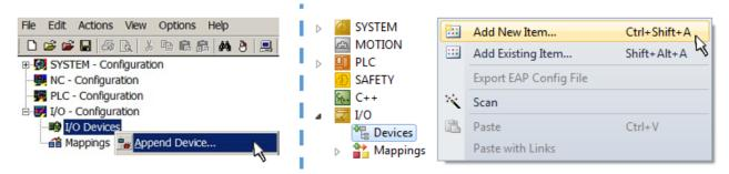
Fig. 91: Append EtherCAT device (left: TwinCAT 2; right: TwinCAT 3)
