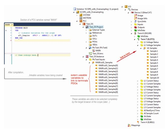
Fig. 143: Representation of a created PLC array variable ("aUI\_Samples") to link with oversampling PDOs of EL3773
