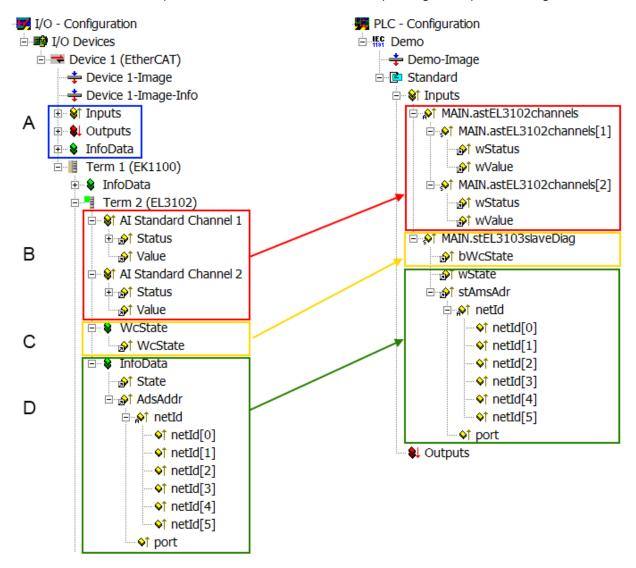
Fig. 133: Basic EtherCAT Slave Diagnosis in the PLC
