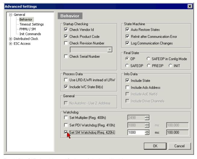
Fig. 13: EtherCAT tab -> Advanced Settings -> Behavior -> Watchdog
