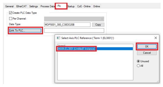
Fig. 72: Linking the structure
