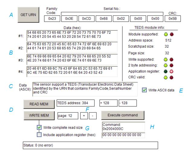
Fig. 190: Visualization of the sample program for TEDS with EL1262-0050 and EL2262
