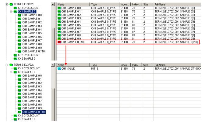
Fig. 169: Automatically calculated array variable (red) in the Scope2
