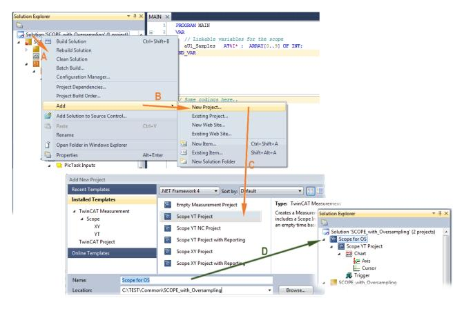
Fig. 142: Adding a Scope project into an already existing project
