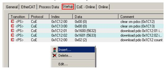
Fig. 16: Startup list in the TwinCAT System Manager
