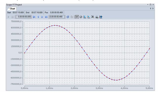
Fig. 151: Example of recording a sine signal with 10 x oversampling at 1 ms measurement cycle time
