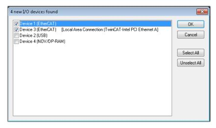
Fig. 58: Automatic detection of I/O devices: selection the devices to be integrated
