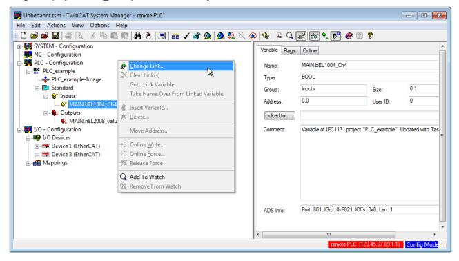
Fig. 46: Creating the links between PLC variables and process objects
