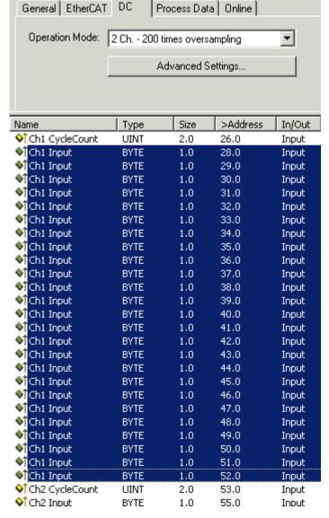
Fig. 174: Select the variables in the terminal with the mouse
