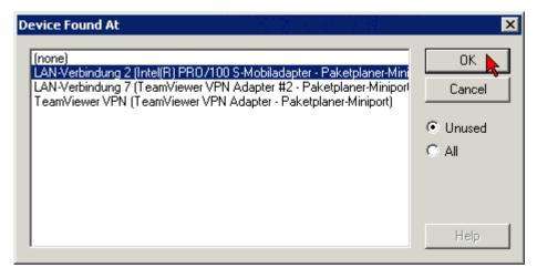
Fig. 182: Selection and confirmation of the Ethernet adapter
