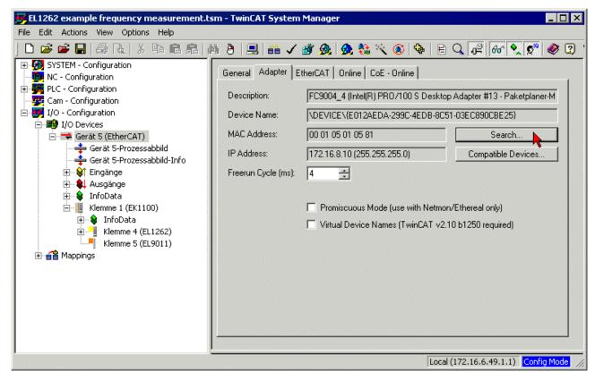
Fig. 181: Searching the Ethernet adapter
