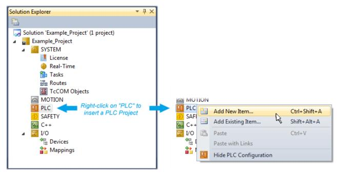
Fig. 61: Adding the programming environment in "PLC"
