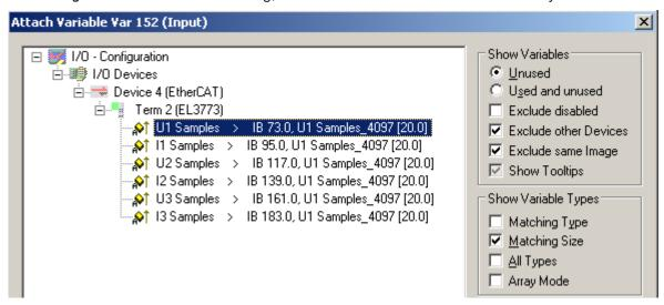
Fig. 160: Array variables of an oversampling terminal
