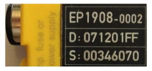
Fig. 6: EP1908-0002 IP67 EtherCAT Safety Box with batch number/ date code 071201FF and unique serial number 00346070
