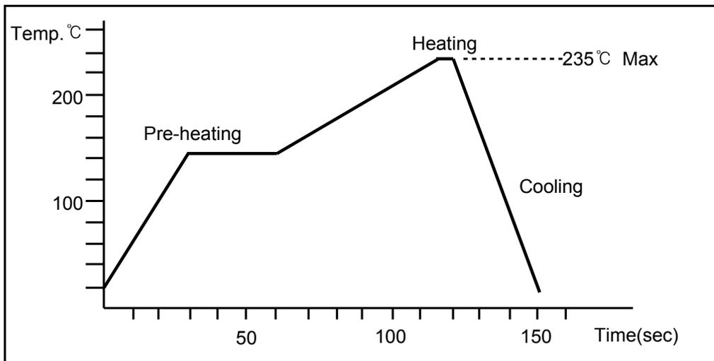
Figure : Typical Temperature Profile of Infrared Reflow Soldering
