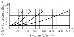
Characteristic curve for differential pressure and flow rate, measured over the check valve  $A \rightarrow B$
