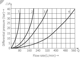
Characteristic curve for differential pressure and flow rate, measured at the throttle position: Throttle fully open (Px=60bar)  $B \rightarrow A$
